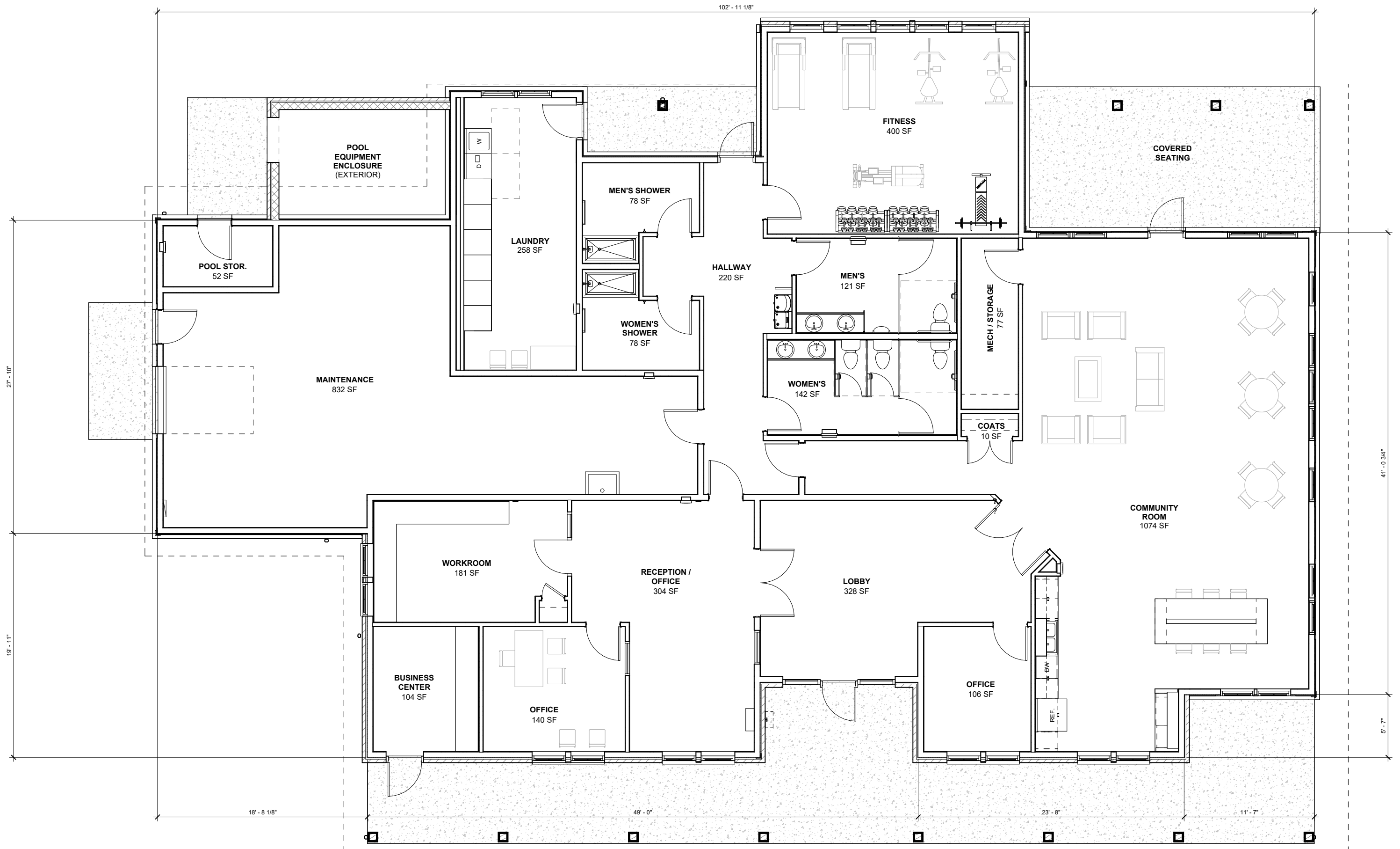
CLUBHOUSE - FIRST FLOOR PLAN SCALE: 1/4" = 1'-0"
